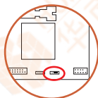
2-1 Clear CMOS Jumper CLR-CMOS
